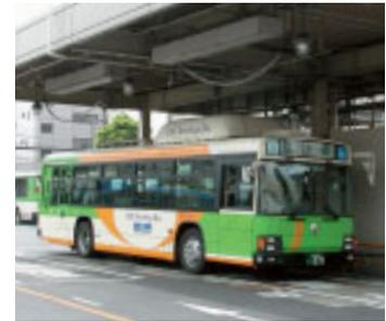
Natural gas vehicles, which produce reduced NOx emissions, include this city bus.
