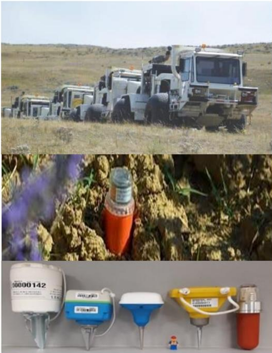
Figure 6-Vibroiseis and Wireless Nodes (Source: Dawson Geophysical Web site)
