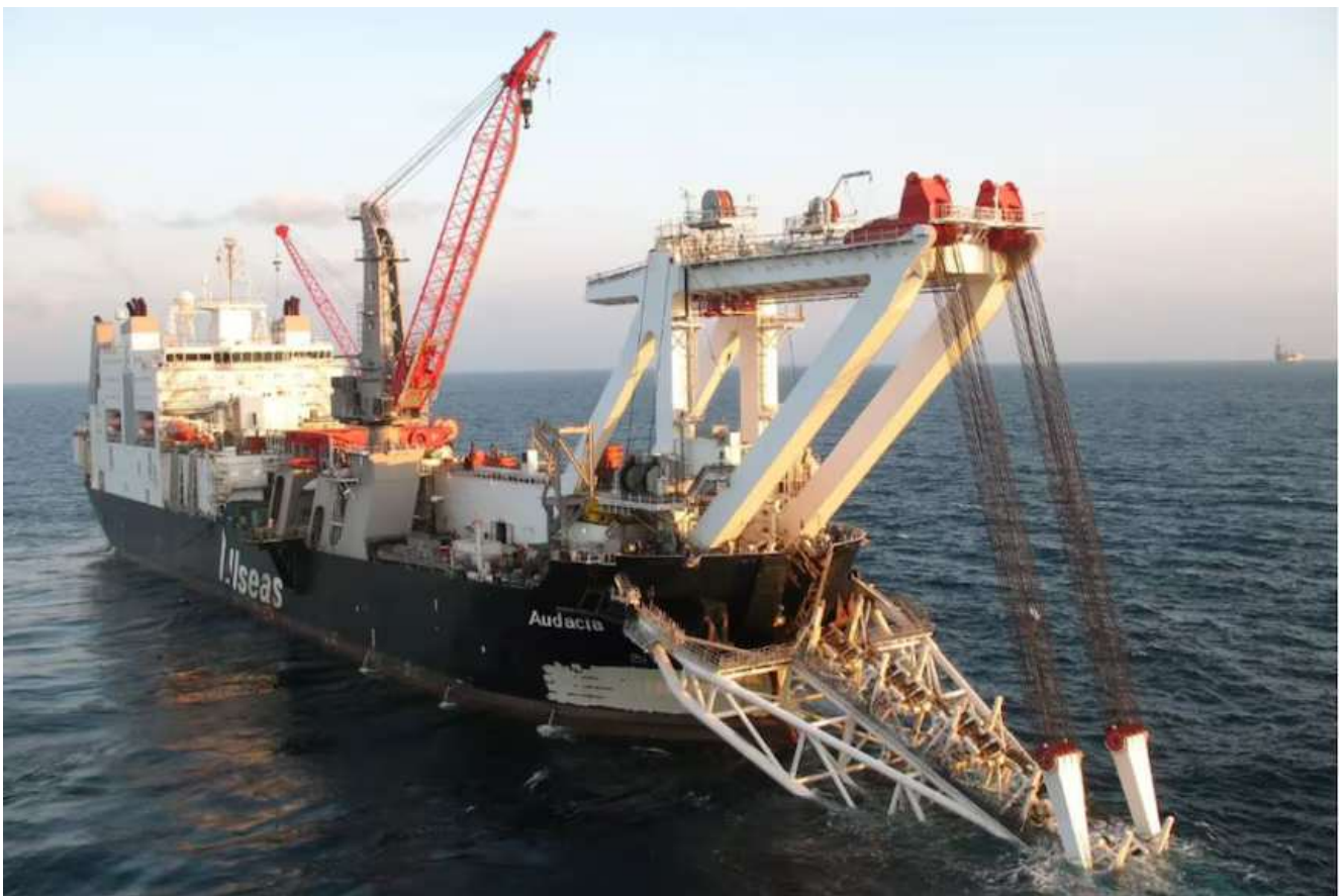
The subsea pipe-laying vessel used by Santos for its Barossa project in the Timor Sea. (Supplied: Santos)
