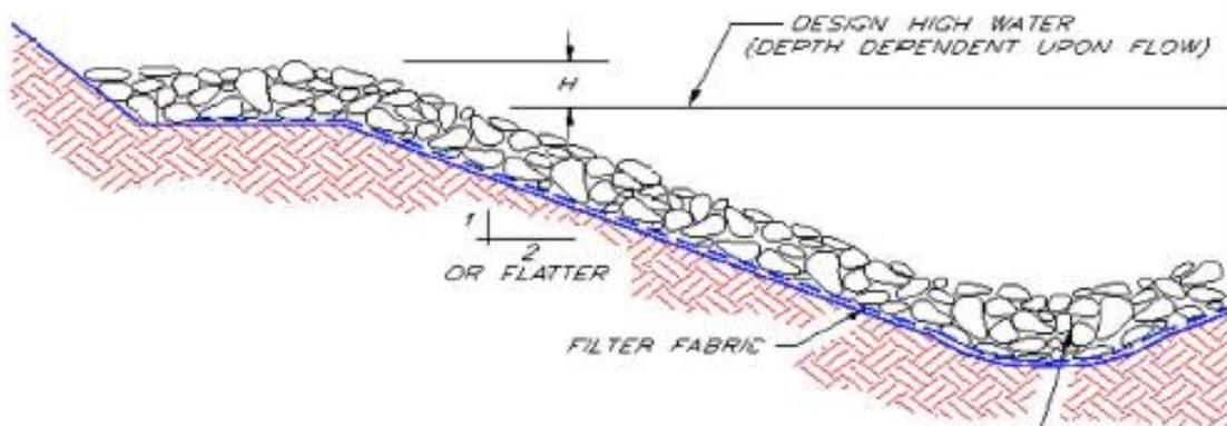
MINIMUM 6" (150mm) THICK LAYER OF 2" (50mm) MINIMUM
