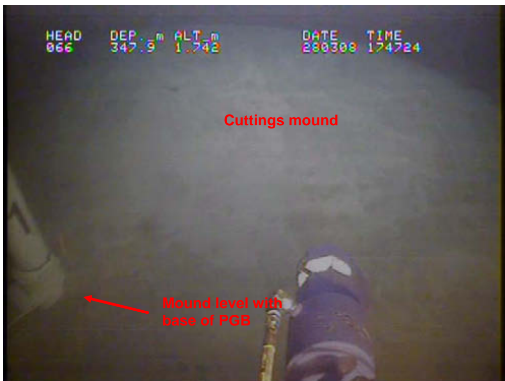
Figure 3.4: Cuttings mound level with the base of PGB (seabed was 2m below PGB prior to drilling)
