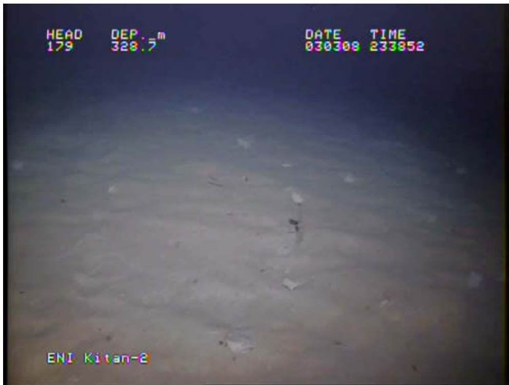
Figure 3.3: View of seabed north of Kitan-2 prior to drilling showing cobbles (probably coral rubble) scattered across the otherwise muddy seabed
