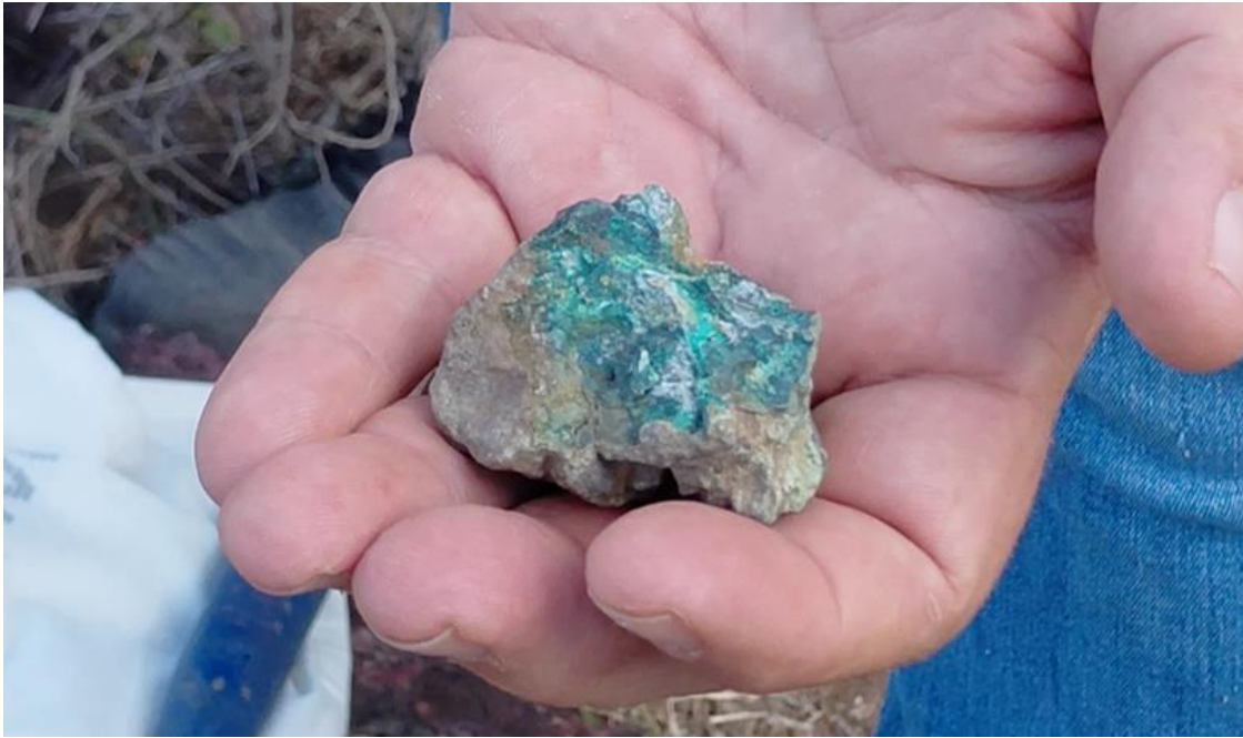
Figure 10: Portion of sample ESR006489, comprised of malachite * (~ 5%) as films on a matrix of magnetite (10-15%), goethite (60-70%) and quartz (20-30%).
