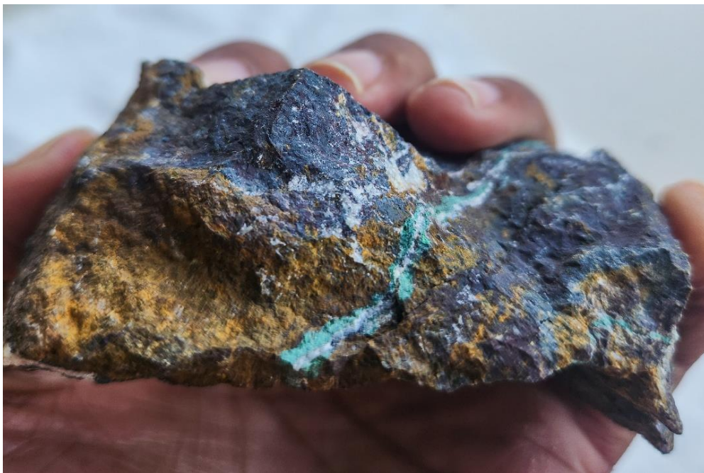
Figure 9: Portion of sample ESR006491 showing quartz veinlet with malachite* note: approx. composition is 1-2% malachite, 30-40% goethite, remainder unknown silicates, chalcedonic silica and trace magnetite.
