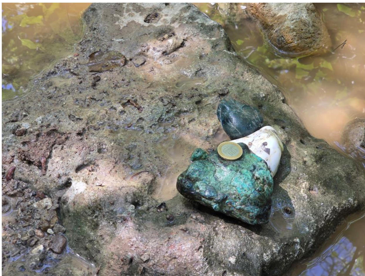
Figure 5: Specimen of oxidised copper-bearing massive sulphide, sampled as ESR006095, which assayed 60.34% Cu
