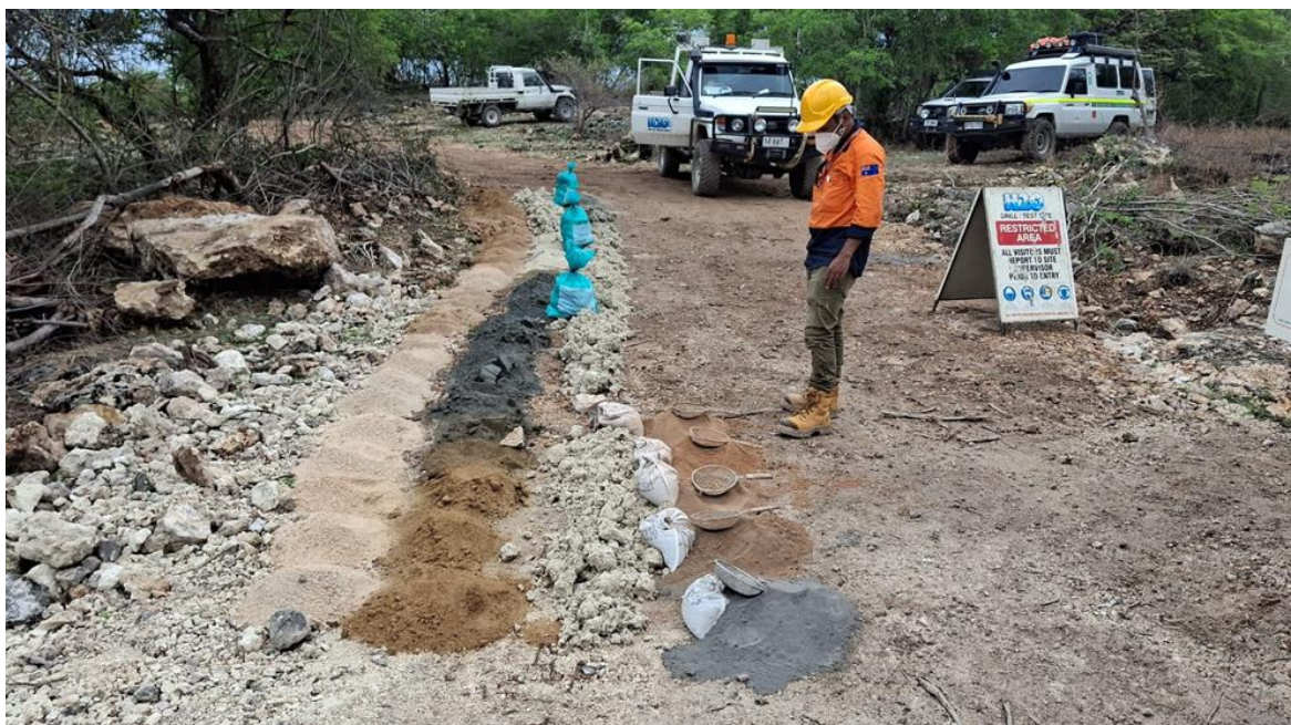
Figure 7: RC drill-cuttings from drill-hole WLR025 laid out in sequence.
