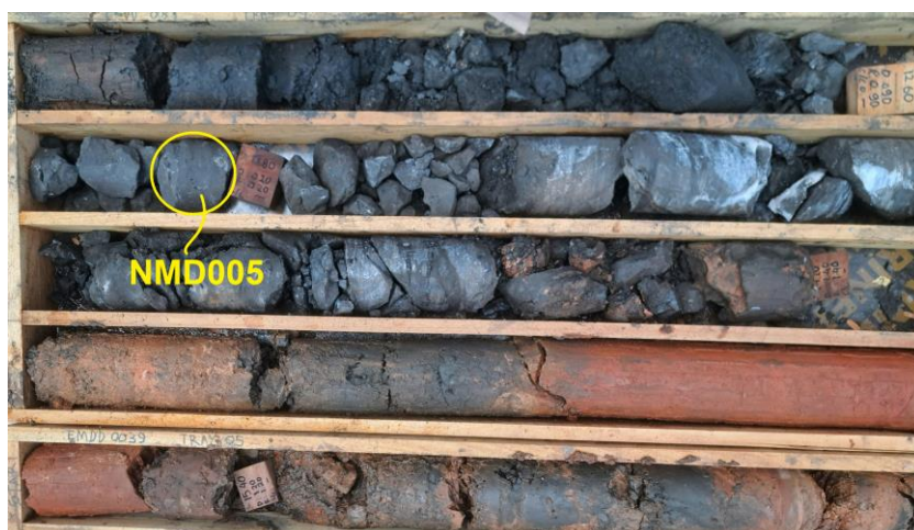
Figure 6: Drill-core from EMDD039 showing the sample (comprised of >95% manganese oxides) collected as NMD005; Refer to Table 2 and Cautionary Statement regarding visual estimates.
