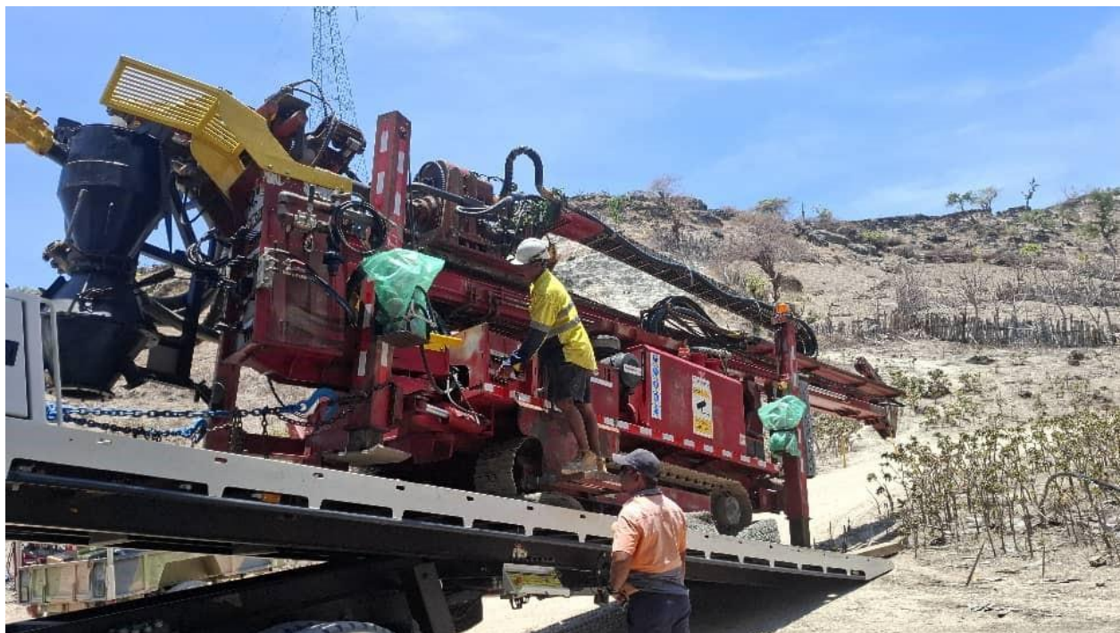
Figure 2. RC drill rig unloading at Werumata staging point in preparation of commencement of drilling
