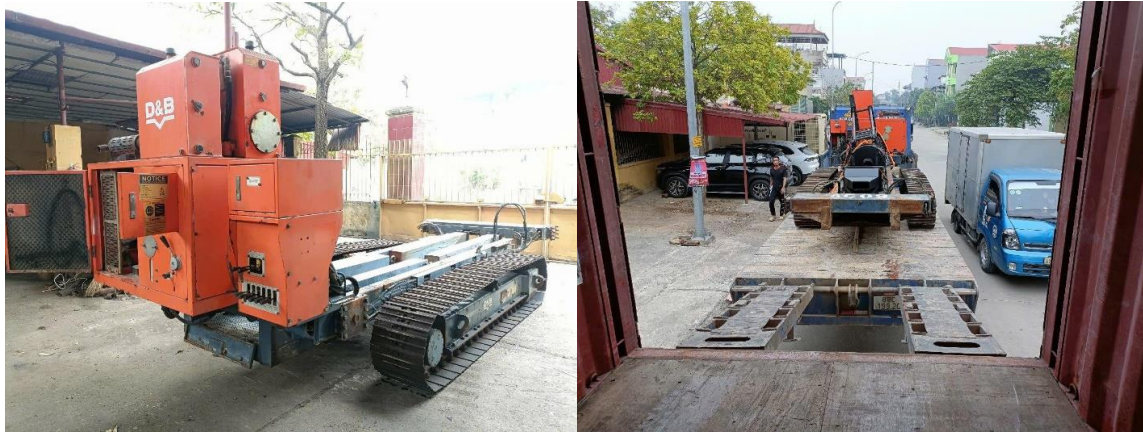
Figure 14: Track carrier and RC sample system from Vietnam being loaded into a sea container for transport to Timor-Leste
