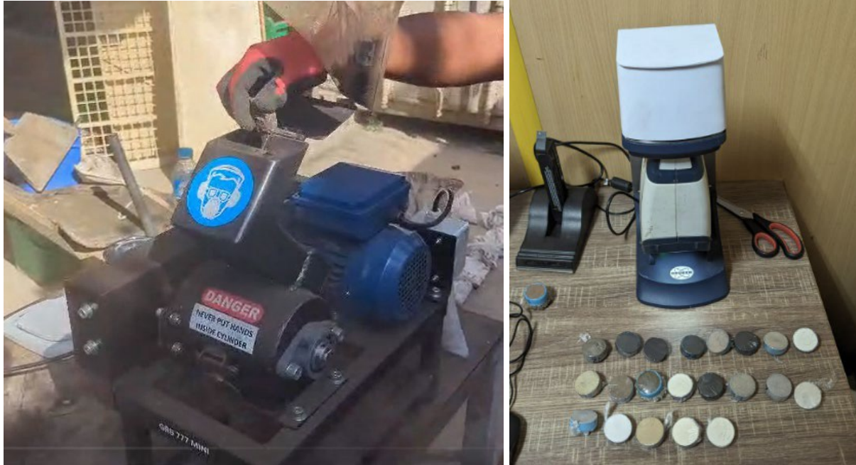
Figure 7: Crusher / Pulveriser and pXRF analysis system set up at Estrella's office in Dili with pulverised samples ready for analysis.
