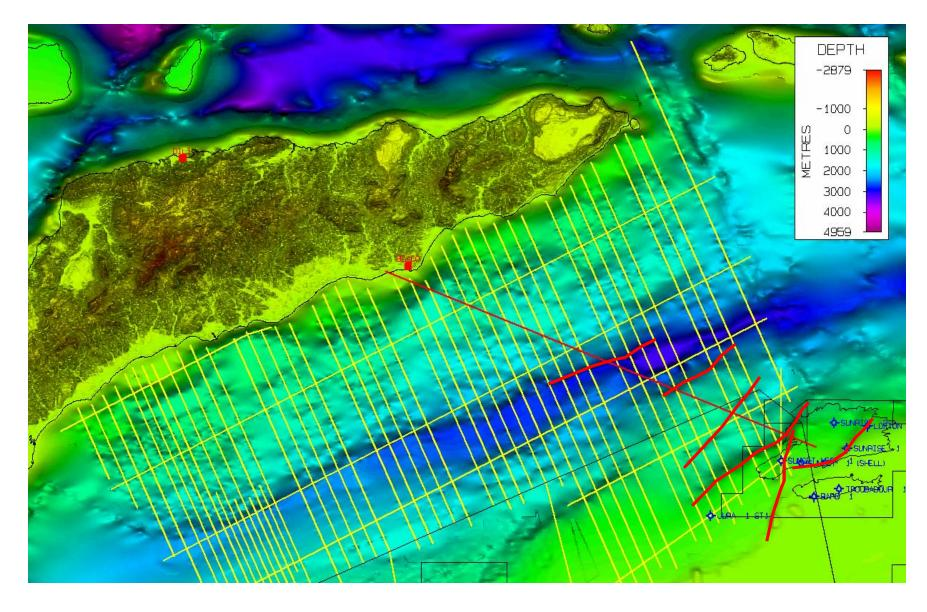
Sunrise Field is adjacent to major faults and topography at seabed, so pipeline routing WILL be affected
