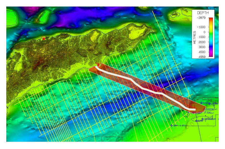
Recommended next steps – 3) Use 1km profiles to define area for detailed swath bathymetry
