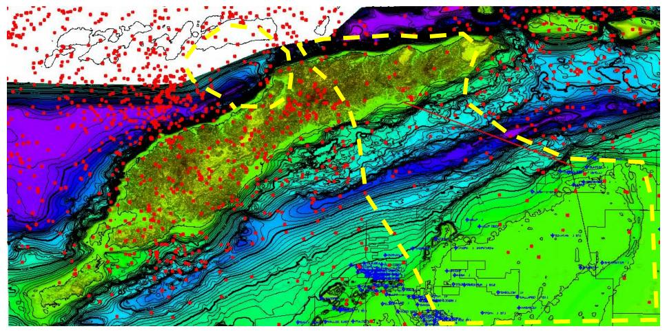
Seismic gaps may either be future major fractures, or could be geologically quiet. A major seismic quiet zone accomodates our pipeline route
