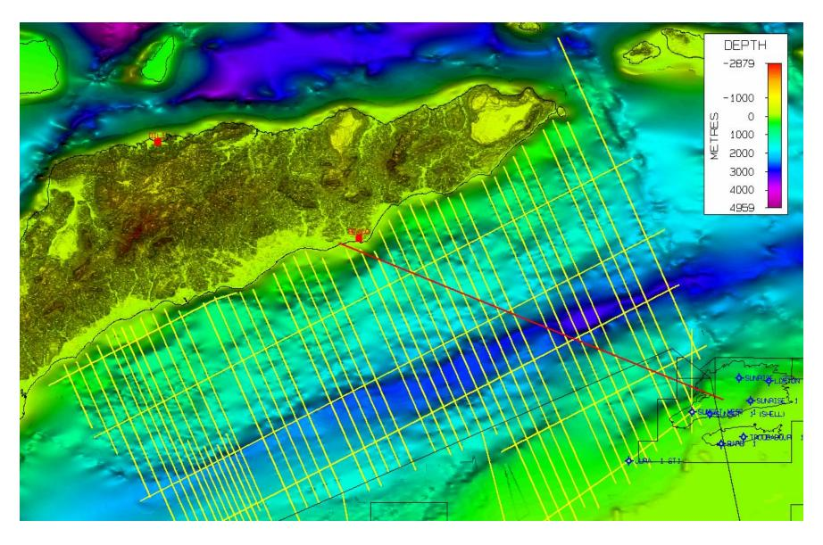
Pipeline Route will cross near deepest part of Trough and over steep slopes.
