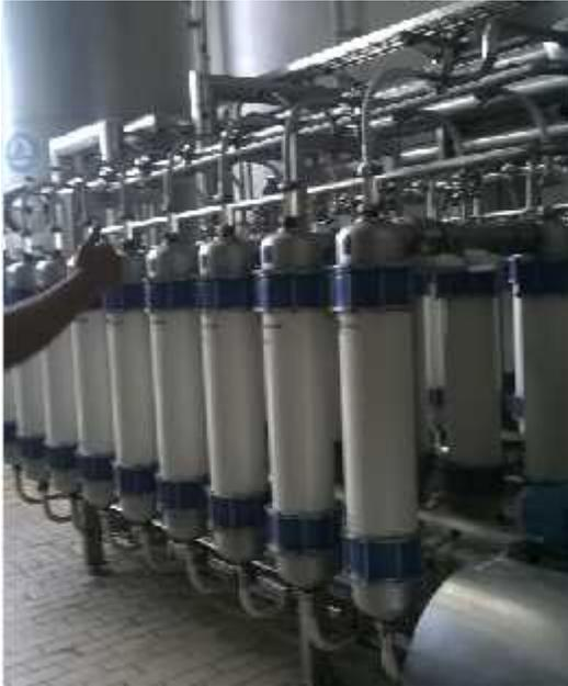
Figure 4.16 Micro-Filtration unit that Filter the Mature Beer
