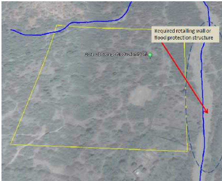
Figure 6.13 Identification of Potential Requirement of Flood Retaining Wall
