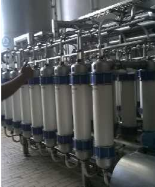
Figure 4.16 Micro-Filtration unit that Filter the Mature Beer
