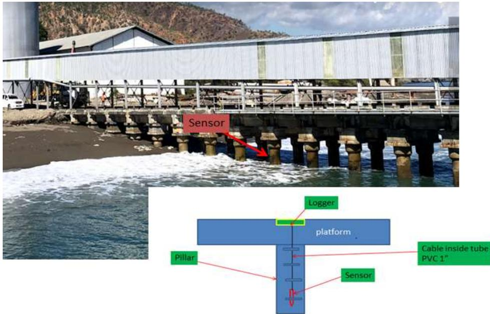
The measurement method is based on the hydraulic pressure that measured by the automatic sensor, installed under existing bridge of the jetty. The water depth, shall be calculated by the following equation, which should be done automatically by the instrument and store the data inside the data logger.
