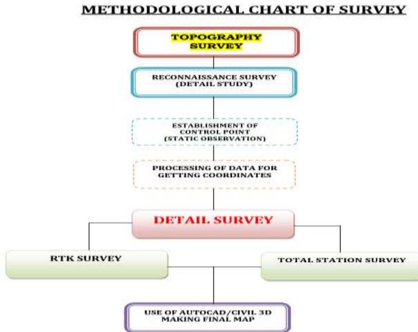
The following figure shows the most common use of differential GPS that uses in the ground survey of topographic data collection.
