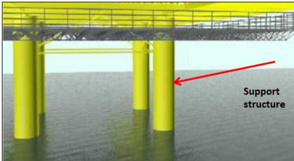
Figure 2.6 Typical Support Structure of Jetty or Above Water Platform
