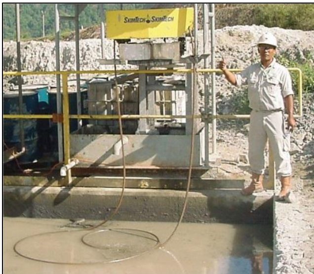
Figure 6.2. Higher-Grade Skimming Machine (Cost US$ 15,000 – US$ 35,000)
