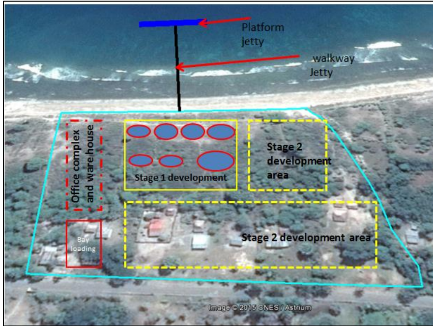
Figure 2.2 Project Boundary and Major Components of Project
