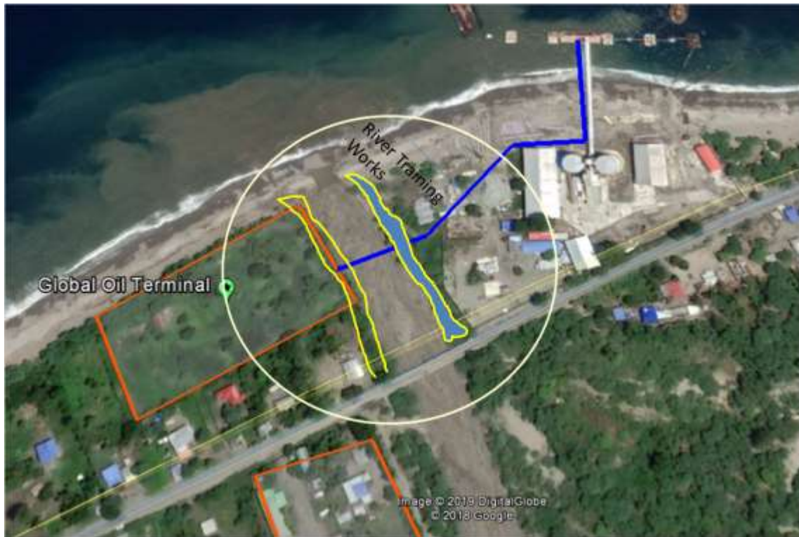
Figure. 7.4 Section of River that need Improvement
